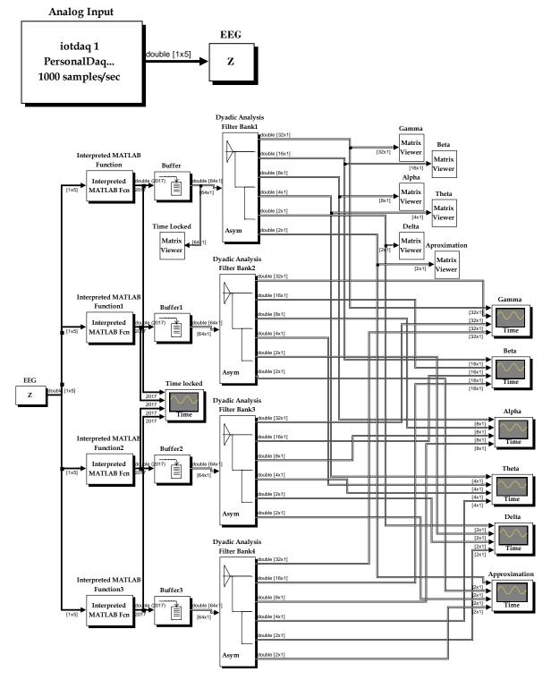
Figure 3. MATLAB Simulink model, importing the data in real-time to Simulink environment, time-lock averaging, and dyadic filter bank wavelet analysis
