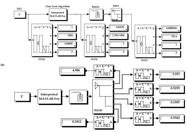
Figure 6. MATLAB Simulink model singular value decomposition of dyadic filter bank
